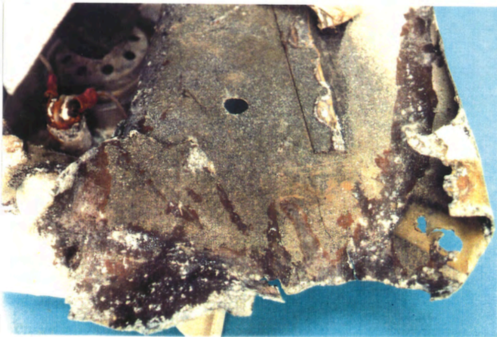
FIG. 72 TORN END SHOWING CORROSION AND DAMAGE
